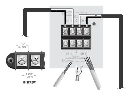
Figure 3.5 Output Connector Wiring (Typical of two channels)
